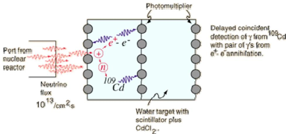
The detector vessel is filled with water in which cadmium chloride is dissolved. The neutrons from the inverse beta decay are captured by cadmium nuclei:
